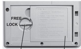
Battery cover lock's handle Battery cover
