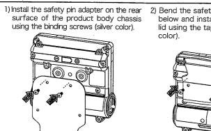
Bend the safety pin adapter from below and install it on the battery lid using the tapping screws (gold color).
