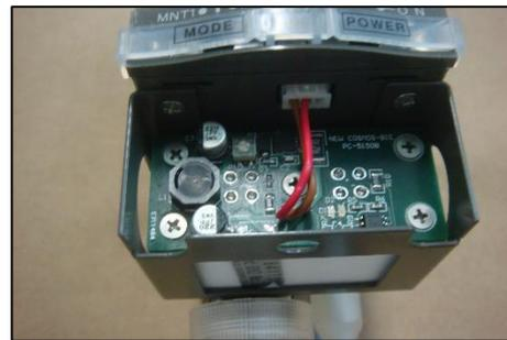
7. Re-fit the pyrolyzer case cover and push the cover lock knob upward. Switch the main unit power ON.
