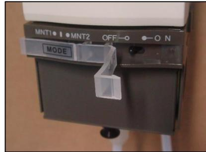
2. Pull the cover lock knob down and release the lock. And after pulling it down further below, pull back the pyrolyzer case cover and remove it.
