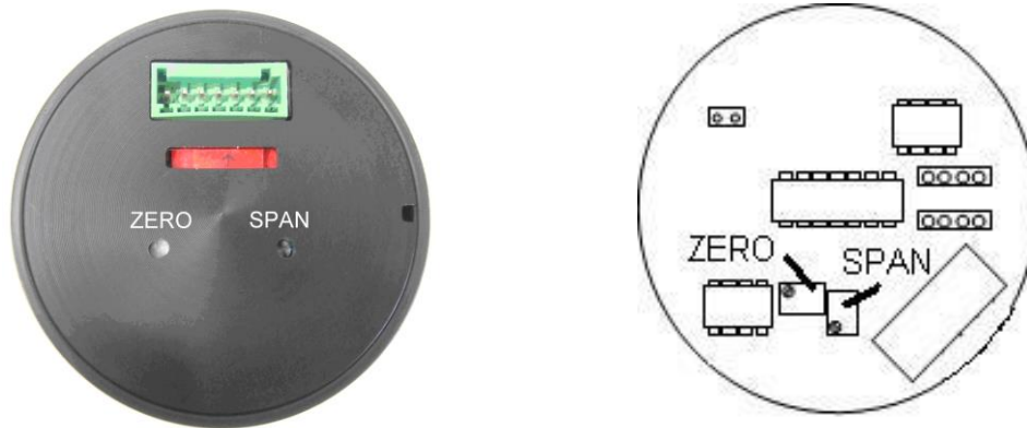
fig. 4.5.3.: Span adjust for different type of transmitter board.
